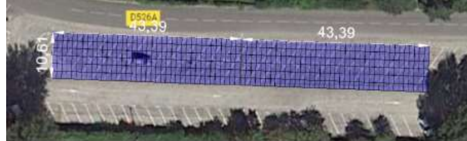
Scenario 1 : Ombrière double - Loyer 1000 €/an Hmax = 4,68 m L = 11,093m
