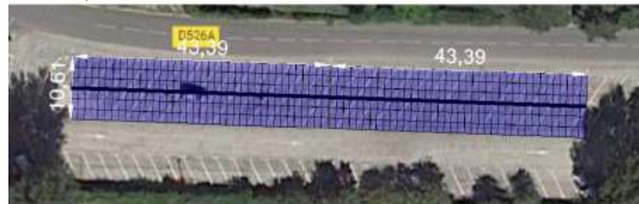
Scenario 2 : Ombrière double papillon - Loyer 300 €/an Hmax = 4,051 m L = 11,463m
